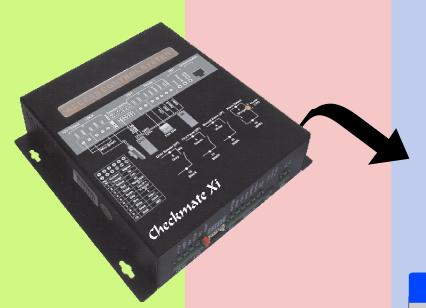
Checkmate Xi is a Competitive single door access controls have 2 kind of communications RS485 or TCP/IP. We put a metal casing and put power supply (12V 4A) Inside to make the cost reduce much. It can connect 2 readers to realize door entry or exit by swiping card and anti pass back.
