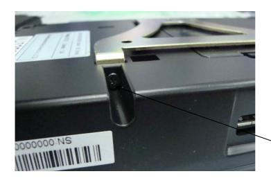
Screw for fixing the rack to the device
